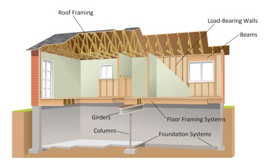
LOAD-BEARING ELEMENTS Examples of load-bearing elements typically covered under the ten year structural warranty.
